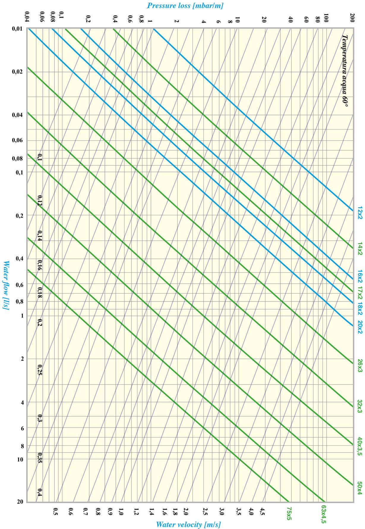
Continuous pressure losses for conveyance of water at 80°C
