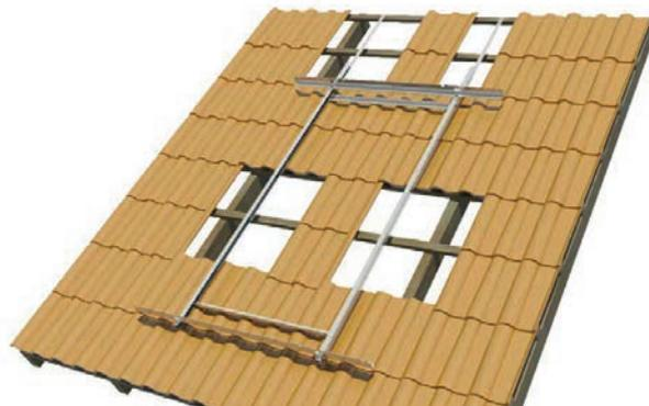
First place the left one, lifting the collector's upper and lower fixing washers (9). When the collector is placed under, we slightly tighten the M8 screws and nuts with the collector's fixing washers (9) in order to temporarily restrain it and easily center it with the system. Place the mechanically tightened unions  $\varnothing 22$  at the collector's edges.
